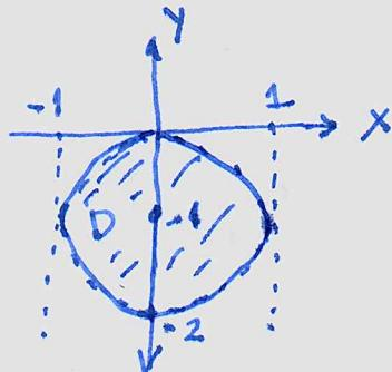
$$\begin{aligned} y &= -1 + \sqrt{1-x^2} \\ \Rightarrow (y+1)^2 &= 1-x^2 \\ \Rightarrow x^2 + (y+1)^2 &= 1 \end{aligned}$$
